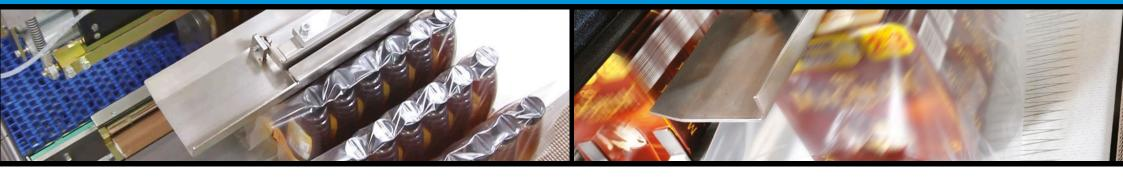
The shrink wrappers in our range are design for heavy usage, 24/7 operation. The standard machines work from two reels of film and are suitable for stable and trayed products, with the servo machine running at up to 30 cycles per minute.
