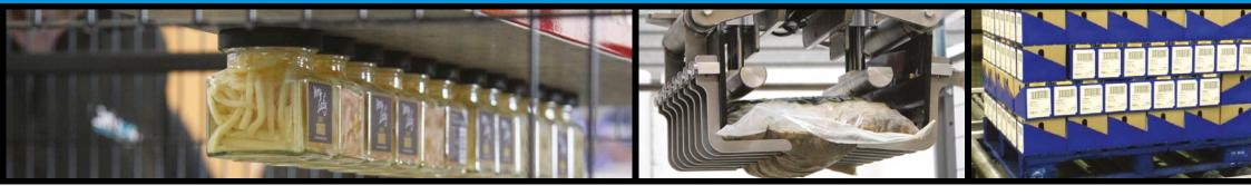
The robot palletiser systems are modular in construction for reliable and flexible palletising solutions. The robotic palletiser can palletise single or multiple products onto multiple pallets, with layer pad, pallet handling and pallet stretch wrapping.
