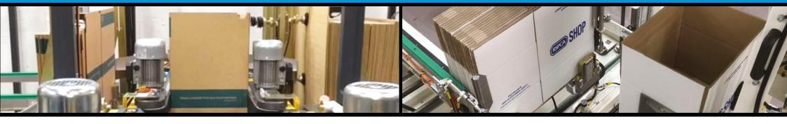
The case/carton erector range work from a flat pre-folded and glued board, and automatically erect into cases/cartons at up to 20 cycles per minute on a single head machine. The machines are designed for easy, repeatable size changing in a compact footprint.
