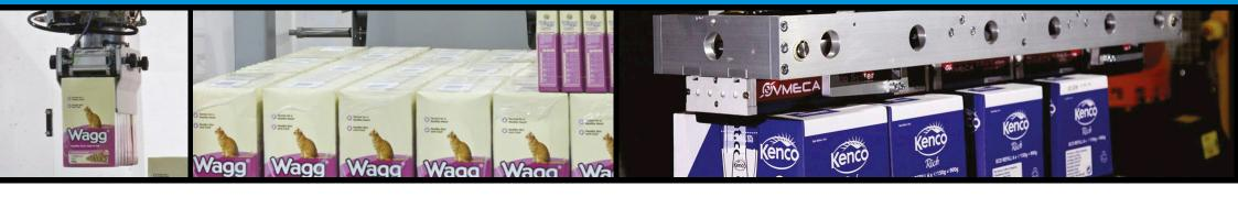
The Compact Gantry Palletisers are designed to meet modern production environments where space is a constraint and the need for potential future expansion is a consideration. Its modular design allows the introduction of pallet conveyors with single and twin pallet and pick positions.
