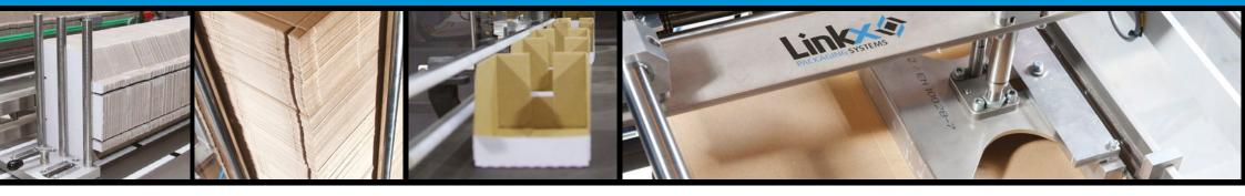
The tray and carton erector range work from a flat die cut board blank and automatically erect a range of trays and cartons at up to 60 cycles per minute on a single head machine.
